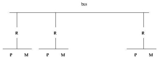
Each P/M/R set here is called a **processing element** (PE). Note that each PE has its own local bus, and is also connected to the global bus via R, the router.
