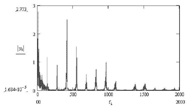
Note that this graph is very "spiky." In other words, even though the reed's waveform includes all frequencies, most of the power of the signal is at a few frequencies which arise from the physical properties of the reed.
