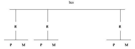
Each P/M/R set here is called a **processing element** (PE). Note that each PE has its own local bus, and is also connected to the global bus via R, the router.
