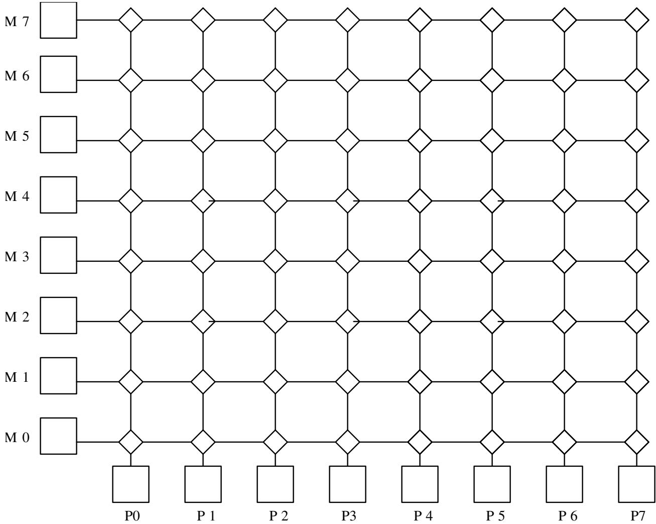
Communication from node to node consists of a packet containing information on both source address (i.e. processor number) and destination address (memory module number). E.g. if P2 wants to read from M5, the source and destination will be 3-bit strings in the packet, coded as 010 and 101, respectively. Note that the source address is needed, since M5 needs to know to which processor it should send its reply.
