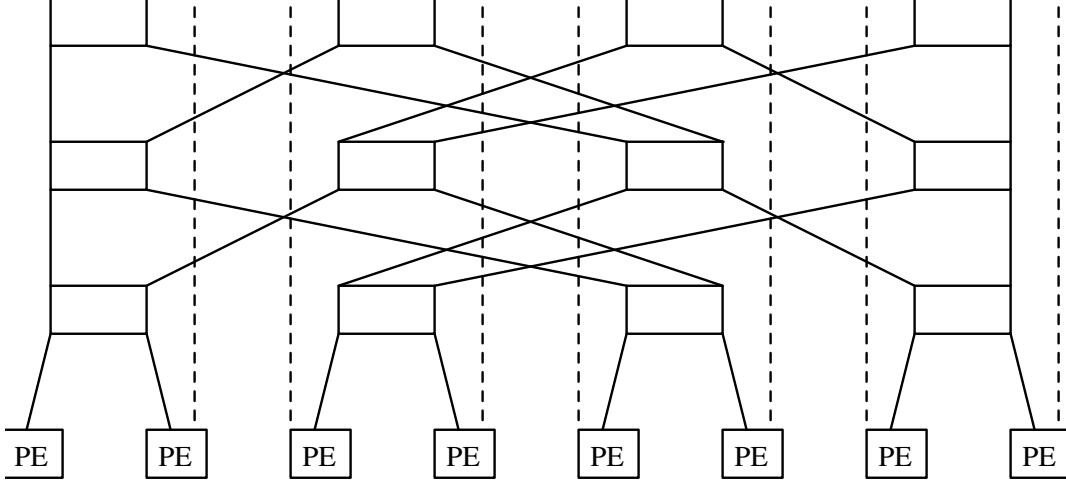
The PEs are processing elements, consisting of a CPU and a memory module. Thus each CPU has a “favorite” memory module, one that it can access quite quickly relative to accessing the other memory modules.<sup>10</sup> But the memory modules still collectively define the address space shared by all the processors, and if a CPU needs to access a “remote” module, it will send a packet through the network.
